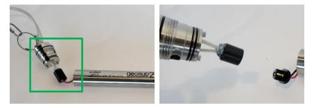
5. Use an appropriate tool to lightly twist and then pull the motor impeller, to remove it. The Geosub 2 assembly/disassembly tool is recommended to avoid damage to the impeller or internal wires.
