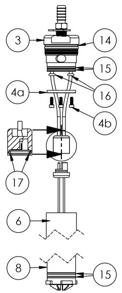
Figure 7-2: Geosub 2 Pump, O-Ring Diagram
