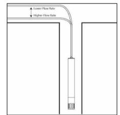
Figure 1-2: Minor Adjustments to Flow Rate
