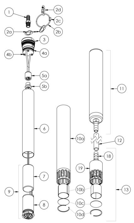
Figure 7-1: Geosub 2 Pump and Drop Tube Assembly
